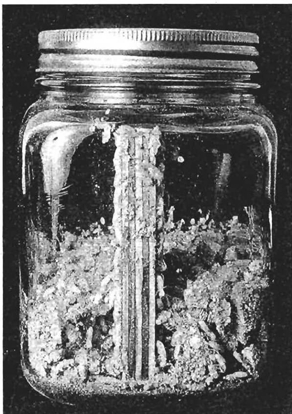
Bioassay used to assess Wellply-treated plywood against the subterranean termite Mastotermes darwiniensis
