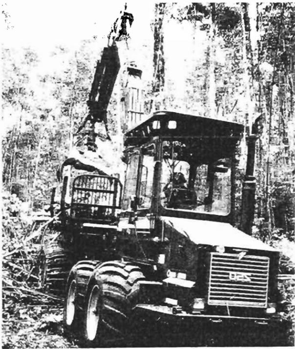
Feller-forwarder equipped with a long-reach crane and grapple saw has the capacity to fell standing trees, crosscut into short (6m) lengths and transport logs to roadside
